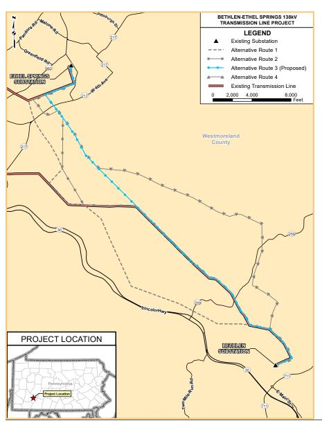
Taking that feedback into consideration, KATCo has selected a proposed route for the new 138-kV transmission line.
