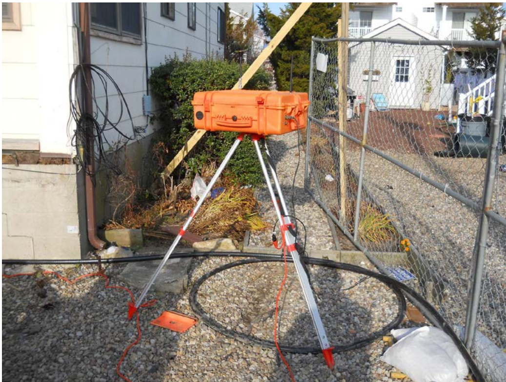
Perimeter Air Monitoring (PAM) Station
