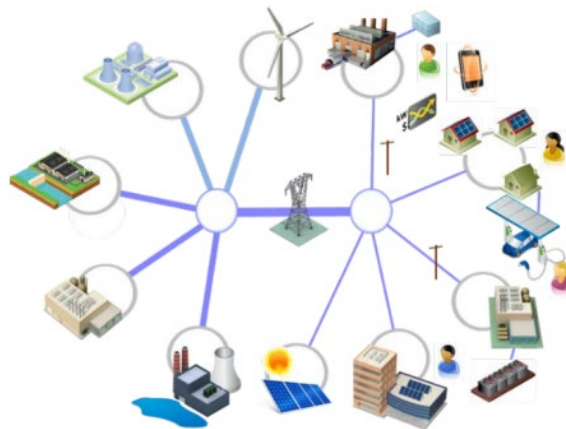
4 Figure 5: Distribution System Increasingly Find More Distributed Energy Resources
